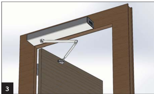
Assembly on the opposite hinge side push version with standard arm page 12
