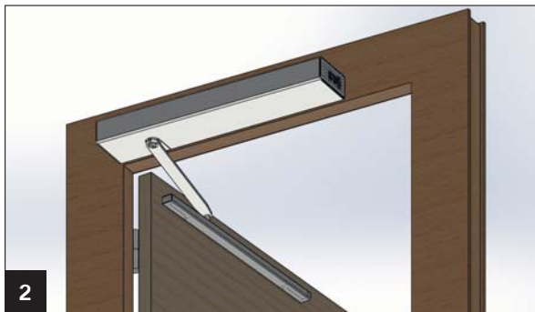
Assembly on the opposite hinge side push version with slide channel page 11
